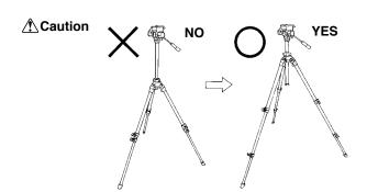
To avoid unnecessary camera vibrations, try to keep the Center Column height to a minimum.
