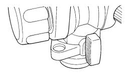
Bubble levels are built-in for vertical and horizontal positioning.
