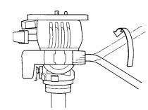
Pan & Tilt Handle can be changed to the left-hand if you reverse it. Please level the Vertical Tilt Lock Knob and then, insert Pan & Tilt Handle from the front. Screw a Handle in the Handle Lock Knob. Tighten the Handle Lock Knob in full by changing the position of a fin part of this knob when the end of screw thread comes.
