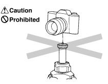
Do not attach camera directly to the threaded post of the Center Column. This may damage both camera and tripod.
