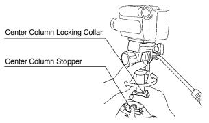
Hold onto the Pan Head with one hand, and loosen the Center Column Stopper and the Center Column Locking Collar with the other hand. Raise or lower Pan Head to desired height, and while maintaining a hold of the Pan Head, tighten the Locking Collar and the Stopper.
