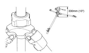
After choosing the desired leg angle, securely push in the Adjustment Lock.
