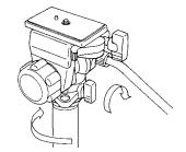
Use the following instructions if you wish to change heads, or attach accessories. First, lock the Panning Lock Knob, then grasp the Pan & Tilt Handle and turn the head, counter-clockwise to loosen.
