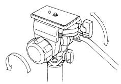
Loosen the Tilting Lock Knob, and the head will tilt back and forth.
