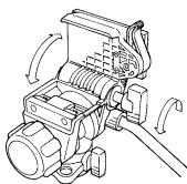
Loosen the Vertical Tilt Lock Knob, and the level can be adjusted.
