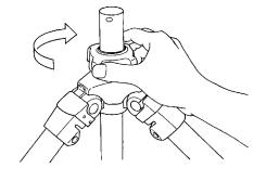
Insert the Center Column from the lower side of Main Body, and tighten the Locking Collar and the Center Column Stopper.
