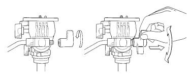
Please remove the Handle Lock Knob and then, insert Pan & Tilt Handle in the axis hole. Please tighten the Knob with your required angle. You can change the position of a fin part of the Knob if you pull it to the front.
