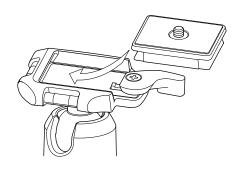
Attach the shoe slid aslant from a Shoe locking lever side. If it attaches, although closed automatically, a Shoe locking lever is further fastened to a lever fixation-side, and is certainly fixed.
