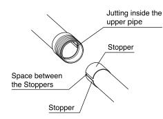
Match the space between the Stoppers and jutting inside the upper pipe when the pipe is connecting.
