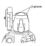
To set vertical camera position, place the Camera platform into U-groove.
