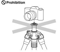
Do not attach a camera directly to the attachment screw of the Center column.
