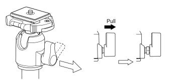
You can change a position of a Ball fixing knob.
