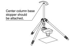
Insert the new replacement Center column through the top, then tighten the Locking collar. Always be sure to return the Center column base stopper back on the bottom of the center column. This prevents the center column pulled out accidentally.
