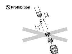
Do not remove the nut and do not take to pieces. If it has been removed, insert it as per the above specification
