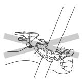
Please do not use an optional Clamp head for a carbon fiber tripod. The pipe may be damaged.
