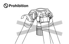
Please do not turn the Center column stopper while a Center column or optional Short center column attached on.
