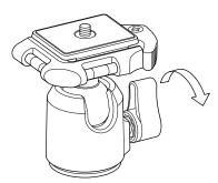
A camera can be moved freely while Ball fixing knob is loosened. Tighten Ball fixing knob when a camera angle is determined.
