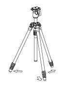
Prevent accidental equipment fall, or tripod tipping over, by making sure all levers, knobs, and handles on the tripod are securely tightened, and that all three legs are opened all the way.
