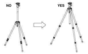
To avoid unnecessary camera vibrations, try to keep the Center column height to a minimum.
