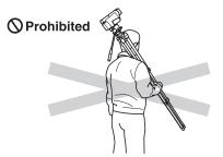
Carrying a tripod with a camera left on can result in unexpected accidents. We therefore, recommend you to remove your camera while carrying the tripod.
