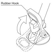
Put the spike of leg-tip on the roller of footpats and hook a rubber hook on the leg-tip.
