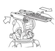
Please remove a camera shoe out behind the head, while pushing a camera mount shoe stopper.
