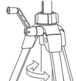
Use the Center Column Tension Adjustment Tube located around the Center Column if you wish to adjust the tension of the Center Column movement.
