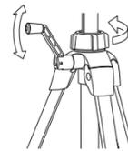
Loosen the Center Column Locking Collar by turning it counterclockwise, and turn the elevation crank handle to raise or lower the center column.
