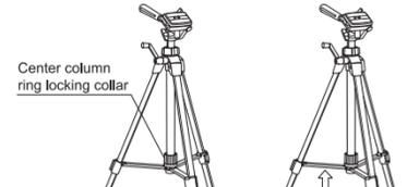
Holding two legs, one in each hand, tilt the tripod on its third leg. Pull the two legs you are holding outward, and all three legs will open at once. Open until the Center Column Ring is seated at the very bottom of the Center Column Cover.
