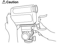
retractable camera positioning pin to holes at the camera side. Then, fix it with mounting wing nut tightly.
