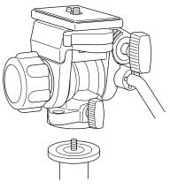
Always remove the pan head when replacing the center column.
