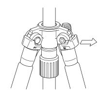
To change the angle of each leg, close the leg slightly, and then pull the leg angle adjustment lock out.
