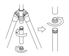
Remove the center column base stopper and then, remove the lower part of center column,
