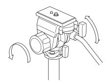
Loosen the tilting lock knob, and the head will tilt back and forth.
