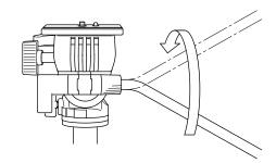
Pan & tilt handle can be changed to the left-hand if you reverse it. Please level the vertical tilt lock knob and then, insert pan & tilt handle from the front. Screw a handle in the handle lock knob. Tighten the handle lock knob in full by changing the position of a fin part of this knob when the end of screw thread comes.
