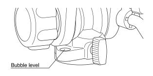
Bubble level is built-in for vertical and horizontal positioning.
