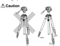
To prevent accidental equipment fall or tripod tipping over, making sure all levers, knobs and handles on the tripod are securely tightened. And all of the three legs are opened all the way.
