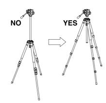
To avoid unnecessary camera vibrations, try to keep the center column height to a minimum.
