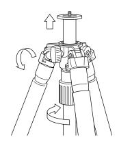
Remove the center column base stopper from the bottom of the center column.
