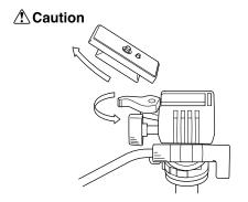
Remove the quick release platform turning the lock lever.
