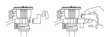
Please remove the handle lock knob and then, insert pan & tilt handle in the axis hole. Please tighten the knob with your required angle. You can change the position of a fin part of the knob if you pull it to the front
