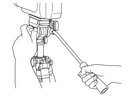
When loosening either the knobs, or the levers, take precaution by keeping a firm grip on the handle until the pan head is locked down.
