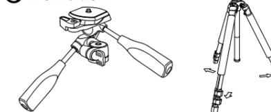
Prevent accidental equipment fall, or tripod tipping over, by making sure all levers, knobs, and handles on the tripod are securely tightened, and that all three legs are opened all the way.
