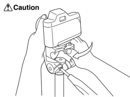
When attaching the camera to the pan head, check to make sure that the quick release platform is engaged in the catch of the pan head before locking the lever.
