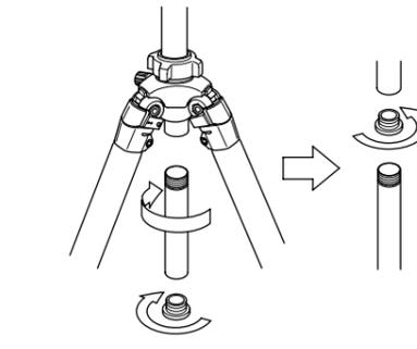
Remove the center column base stopper and then, remove the lower part of center column. Put the center column base stopper on the upper part of center column.
