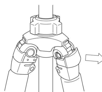
To change the angle of each leg, close the leg slightly, and then pull the leg angle adjustment lock out. There is a choice of two other angle positions.
