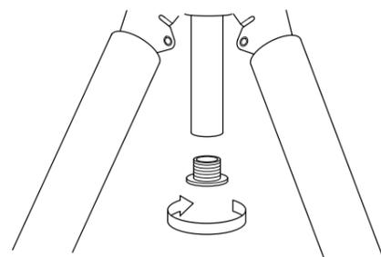
Remove the center column base stopper turning to the way arrow.
