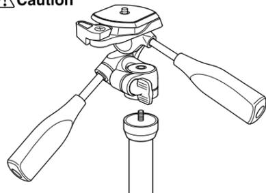
Always remove the pan head when replacing the center column.
