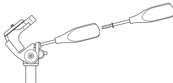
Remove the vertical tilt handle from the pan head, and screw into the back of the pan & tilt handle. Make sure the washer ring on the thread stays on with the handle.
