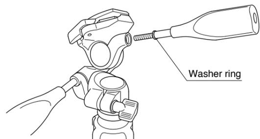
Check to see that there is a washer ring on the shaft of the vertical tilt handle, and then insert the shaft into the threaded hole located on the right side of the pan head. Screw handle all the way in until secure.
