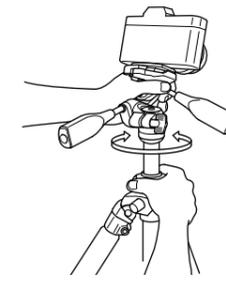
Hold onto the pan head with one hand, and loosen the center column locking collar with the other hand. Raise or lower pan head to desired height, and while maintaining a hold of the pan head, tighten the locking collar.
