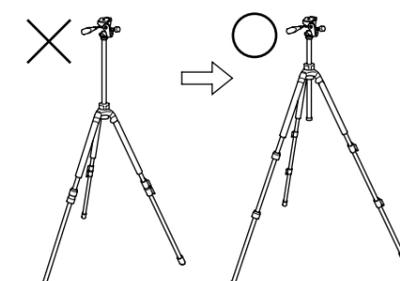
To avoid unnecessary camera vibrations, try to keep the center column height to a minimum. Also use the larger legs first, when extending the legs.
