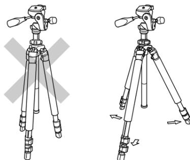
Be sure to open all three legs completely in order to prevent camera shakes, or accidental tip overs caused by unstableness.
