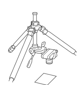
By inverting the center column, it is possible to do copy, and close up work.
