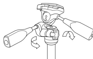
Use the following instructions if you wish to change heads, or attach accessories. First, lock the panning lock knob, then grasp the pan, or vertical tilt handle and turn the head, counter-clockwise to loosen.
