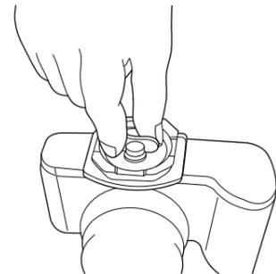
Align the length of the platform along the base of the camera body, and securely tighten the mounting wing nut.
