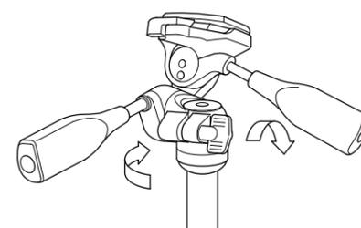
Set the new head, or accessory on the tripod's threaded post, and turn clockwise until it comes to a stop. Tighten the panning lock knob and turn clockwise slightly more.
