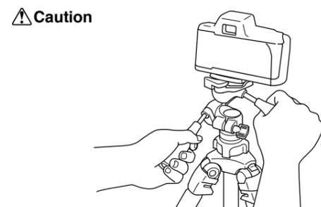
When loosening either the pan & tilt handle, or the vertical tilt handle, take precaution by keeping a firm grip on the handle until the pan head is locked down.
