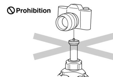
Do not attach camera directly to the threaded post of the center column. This may damage both camera and tripod.
