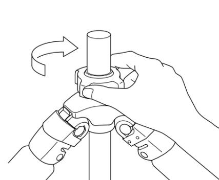
Insert the center column from lower side of main body, and tighten the locking collar and the center column stopper.
