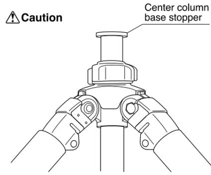
Make sure to re-attach the center column base stopper, in order to prevent the center column from falling out.
