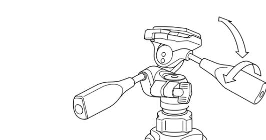
Loosen the vertical tilt handle, and the level can be adjusted.
