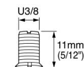
On this tripod, please buy thread adapter set when the pan head that there are large screw (U3/8) tripod installation screws is attached.
