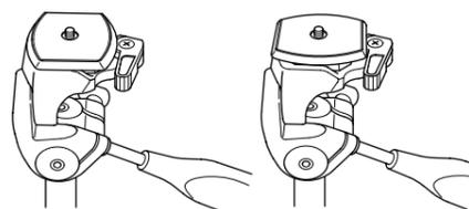
The quick release platform can be attached to the camera body in either directions (along the length, or along the width).□ This feature facilitates your camera set up into the vertical position, simply by the turn of one of the tilt handles.
