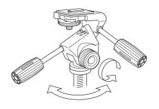
2. Loosen the panning lock knob, and the head will rotate.
