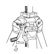
Raise the crank handle into position by pulling out on the knob to lock it into place.
