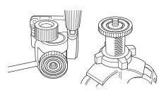
The head is installed by screwing it onto the center column's 3/8" threaded post socket hole.
