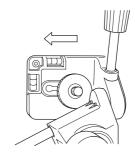
2. Remove the camera mounting screw through the large end of the mounting track. It's a good idea to tighten the camera locking knob when a camera is not attached to prevent loss of the mounting screws.
