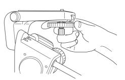
2. Lock the camera tightly with the knurled camera locking knob.
