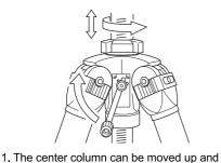
down by turning the clank handle. The center column tension adjustment nut adjusts the tightness of the column and helps The lower center column tension adjustment prevent vibration. nut is used when necessary to adjust the tight-
