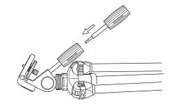
The vertical tilt handle can be reset inside the pan & tilt handle by screwing from rear of the handle as shown here.
