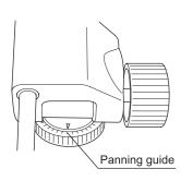
A rotating scale at the base of the head makes it easy to set exact shooting angle. To begin, set the mark at the base of the head on "0".
