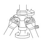
Adjustment of the center column play can be accomplished by locking a screw with the enclosed allen wrench.
