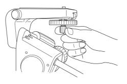
1. Hold the camera firmly, and turn the camera mounting screw to engage the threads.
