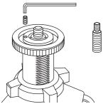
1. The threaded posts on each end of the center column are both reversible, 1/4" on one end and 3/8" on the other.
