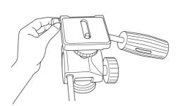
1. Both 1/4" and 3/8" camera mounting screws are supplied.
