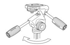
Loosen the panning lock knob and rotate the base of the head clockwise to screw it tightly onto the center column.
