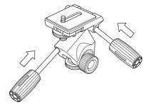
The pan handles are installed as shown with the long handle on the left, for pan and tilt movement; the short on the right, for vertical tilt. If you prefer to have it the other way around, the tripod will function perfectly.
