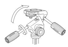
1. Loosen the pan & tilt handle, and the head will move freely front to rear.
