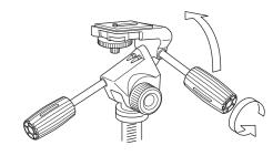
3. Loosen the vertical tilt handle and the level can be adjusted.
