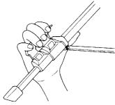
Flip up the Leg lock lever to extend or shorten any of the individual leg sections to the desired length, and press the leg lock lever flush against the lea to lock.
