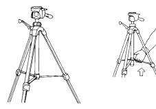
Holding two legs, one in each hand, tilt the tripod on its third leg. Pull the two legs you are holding outward, and all three legs will open at once. Open until the Center column ring is seated at the very bottom of the Center column.
