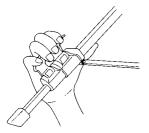
Flip up the Leg Lock Lever to extend or shorten any of the individual leg sections to the desired length, and press the Leg Lock Lever flush against the Leg to lock.
