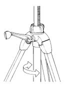
Use the Center Column Tension Adjustment Tube located around the Center Column if you wish to adjust the tension of the Center Column movement.
