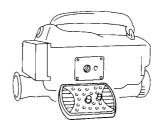
For video cameras, match the Camera Positioning Pin of the Platform to the corresponding hole beneath the camera, and then tighten screw into tripod socket with a coin. Replacement Quick Release Platform for the U 8000 is available.
