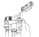
To remove the Quick Release Platform from the Pan Head, turn Quick Release Lock Lever counterclockwise, and lift Platform out at an angle from the side closest to the lever.
