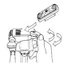
Return Quick Release Platform back onto the Pan Head by inserting at an angle from the side closest to the Quick Release Lock
