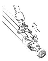
Remove the mid-level spreader sliding each attachment point in the direction of the arrow shown in this diagram. Do this to all legs to completely remove the spreader.
