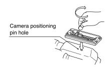
Attach the camera plate by matching it to a tripod mounting screw on the your video camera. If you video camera has a camera alignment pin
