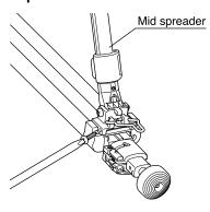
Remove the mid-level spreader when using the tripod with a dolly (sold separately).
