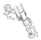
Loosen the Leg lock lever (Lower) to extend or shorten.
