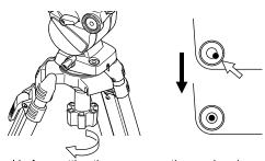
Adjust the level before putting the camera on the pan head.
