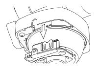
Pull out the LED unit but be careful not to pull out the unit by force, doing so may result breaking the unit.
