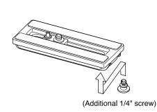
If needed, plase attach it from the back of the long hole of a camera shoe.
