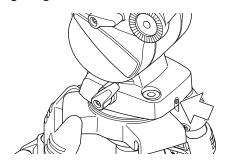
When the LED light button is pushed, a light in the level turns on for approximately 20 seconds.
