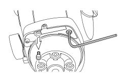
Remove the 2 hex screws on the bottom of the pan head with the included Allen wrench.
