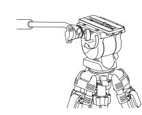
Tighten a tilt lock lever. Loosen a shoe lock lever turning in the direction of an arrow.
