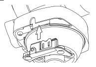
Re-confirm that the battery is properly installed. Put the LED unit back into the pan head and reinstall the 2 hex screws.
