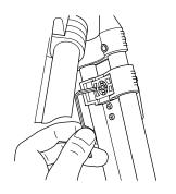
The strength of a lever can be adjusted using an attached Allen wrench (2.5mm width) in the reverse-side of Leg lock lever (Upper).
