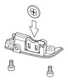
Install a battery model CR1220 with in the correct direction of the battery contacts.
