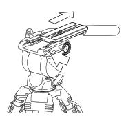
Please remove a camera shoe out behind the head, while pushing a shoe stopper.
