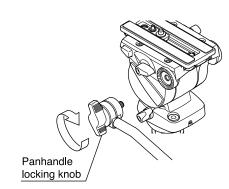
Thrust a pan & tilt handle lightly into the head side by the panhandle locking knob, and adjust to a favorite angle. Please thrust firmly and fix.
