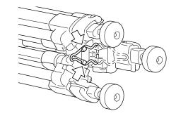
The legs can be locked in the closed position by using the metal hook behind the middle stage.
