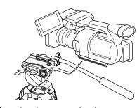
Please insert a camera shoe in a camera plate from the direction of an arrow to back pushing a shoe stopper. If a shoe stopper is released, a camera shoe stops releasing. Please fix a shoe lock lever in total in the good position of
