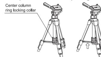
Holding two legs, one in each hand, tilt the tripod on its third leg. Pull the two legs you are holding outward, and all three legs will open at once. Open until the Center Column Ring is seated at the very bottom of the Center Column Cover.
