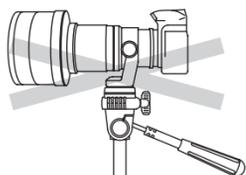
This product has been designed to handle equipment weighing under 1.5 kg (3 lbs 5 oz). Do not overload.
