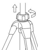
Loosen the Center Column Locking Collar by turning it counterclockwise. Raise the Center Column to the desired height and lock in place by turning the collar clockwise.
