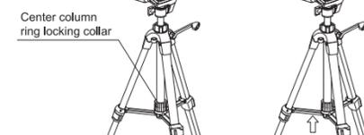
Holding two legs, one in each hand, tilt the tripod on its third leg. Pull the two legs you are holding outward, and all three legs will open at once. Open until the Center Column Ring is seated at the very bottom of the Center Column Cover.
