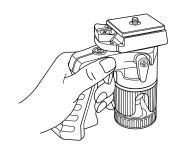
It moves when the Grip is grasped, and pull the Trigger. The Skirt also rotates. If the Trigger is released, it locks.
