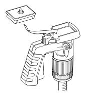
Attach the plate slid aslant from the Plate locking lever. If will be closed automatically after attaching.
