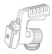
The ball head can be inclined up to 90 degrees to the direction of the Skirt of U-ditch. You can get any angles if you use the rotation of the Skirt and the Camera platform.
