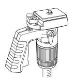
Fasten the plate locking lever to the side of lever fixation. It will be certainly fixed.
