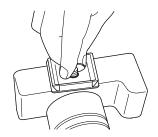
Turn the Camera mounting screw knob and fix firmly.
