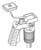
Remove the Quick release plate turning the lock lever.
