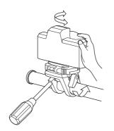
When you unlock the camera platform locking knob, raise the knob it to the vertical "release" position.
