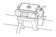
To remove the quick release plate, turn the quick release plate locking lever.
