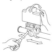
When you unlock the handle, your camera is free to move up and down. When the pan & tilt handle is unlocked, you can pan & tilt simultaneously.
