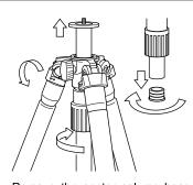
Remove the center column base stopper from the bottom of the center column.
