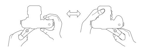
The position of the grip can be freely chosen as the camera platform rotates. Please fix the camera platform with the locking lever when you decide your required position.
