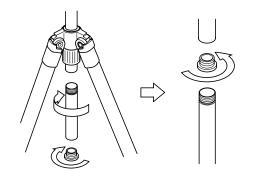
Remove the center column base stopper and then, remove the lower part of center column
