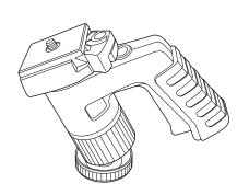
The ball head can be inclined up to 90 degrees to the direction of the skirt of U-ditch. You can get any angles if you use the rotation of the skirt and the camera platform.
