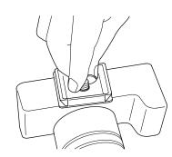
Turn the camera mounting screw knob and fix firmly.
