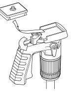
Remove the quick release plate turning the quick release plate locking lever
