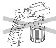
In this case, please do not put the quick release plate locking lever back by force as it has been stood by the stopper.
