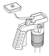
Attach the plate slid aslant from the quick release plate locking lever. It will be closed automatically after attaching.
