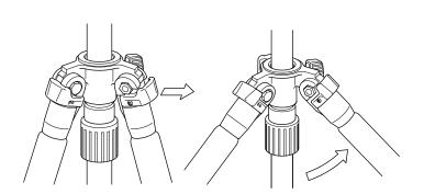
To change the angle of each leg, close the leg slightly, and then pull the leg angle adjustment lock out.
