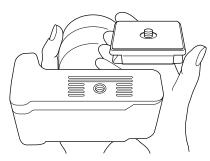
Insert the camera mounting screw of the plate in the place of the tripod attachment screw of your camera.
