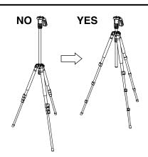
To avoid unnecessary camera vibrations, try to keep the center column height to a minimum.
