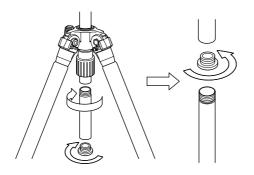
Remove the center column base stopper. Then remove the lower part of center column
