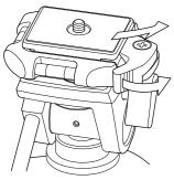
To remove the quick release plate, turn the quick release plate locking lever.
