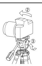
2.Turn your camera to the side.3.Tighten camera platform locking knob.
