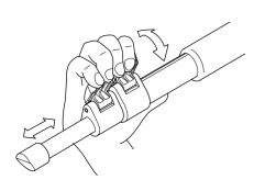
Flip up the leg lock lever to extend or shorten any of the individual leg sections to the desired length and press the leg lock lever flush against the leg to lock.
