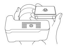
Insert the camera mounting screw on the quick release plate in the place of the tripod attachment screw of your camera.
