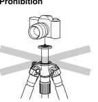
Do not attach camera directly to the threaded post of the center column.
