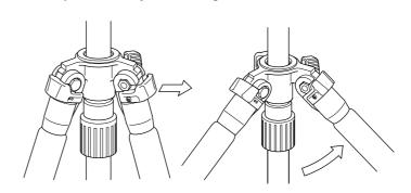
To change the angle of each leg, close the leg slightly. Then pull the 3-position leg angle adjustment locks. There is a choice of two other angle positions.
