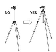
To avoid unnecessary camera vibrations, try to keep the center column height to a minimum.
