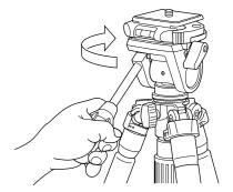
Set the new head or accessory on the tripod's threaded post. Turn clockwise until it comes to a stop.
