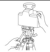
When you unlock the camera platform locking knob, raise the knob it to the vertical "release" position. The camera can be free to rotate.
