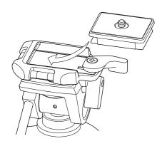
To attach the plate, slide into quick release plate slantways. If will be closed automatically after attaching.
