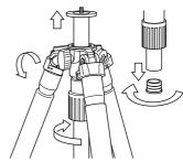
Remove the center column base stopper from the bottom of the center column.
