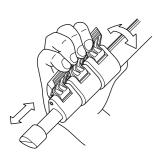
Flip up the leg lock lever to extend or shorten any of the individual leg sections to the desired length and press the leg lock lever flush against the leg to lock.
