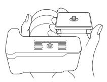
Insert the camera mounting screw of the quick release shoe in the place of the tripod attachment screw of your camera.
