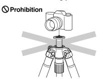
Do not attach a camera directly to the attachment screw of the center column.
