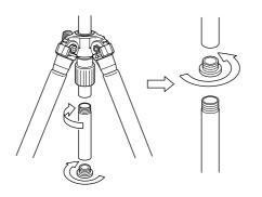
Remove the center column base stopper and then, remove the lower part of center column,
