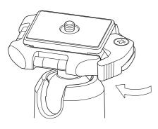
Fasten the shoe locking lever to the side of lever fixation. It will be certainly fixed.
