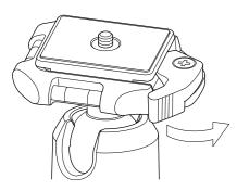
Remove the quick release shoe turning the shoe locking lever.
