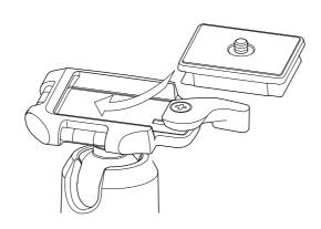
Attach the shoe slid aslant from the shoe locking lever. If will be closed automatically after attaching.
