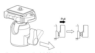
You can change a position of a ball fixing knob.
