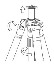
Remove the center column base stopper from the bottom of the center column.
