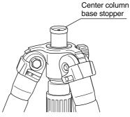
Insert the new replacement center column through the top, and tighten the locking collar.
