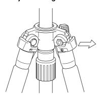
To change the angle of each leg, close the leg slightly, and then pull the leg angle adjustment lock out.
