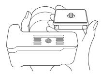
Insert the camera mounting screw on the quick release plate in the place of the tripod attachment screw of your camera.
