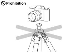
Do not attach a camera directly to the attachment screw of the center column. This may damage both your camera and tripod.
