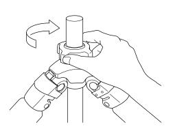
Insert the center column from lower side of main body, and tighten the locking collar and the center column stopper.
