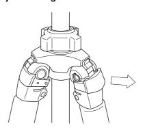
the leg angle adjustment lock out.
