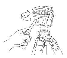
Set the new head or accessory on the tripod's threaded post. Turn clockwise until it comes to a stop.
