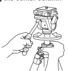
Hold the pan head with one hand Loosen the center column stopper and the center column locking collar with the other hand. Raise or lower pan head to desired height. While maintaining a hold you desired height of the pan head, tighten the locking collar and the
