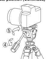
4.Loosen pan & tilt handle for your camera to get the front. 5. Turn the whole of pan & tilt handle.
