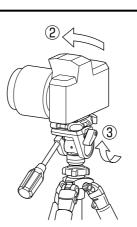
2.Turn your camera to the side. 3. Tighten camera platform locking knob.
