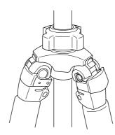
To change the angle of each leg, close the leg slightly and pull the leg angle adjustment lock out.
