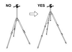
To avoid unnecessary camera vibrations, try to keep the center column height to a minimum. Also use the larger legs first when extending the legs.
