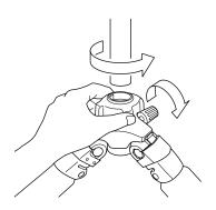
Loosen the center column stopper and the locking collar, and then pull out the center column.
