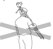
Carrying a tripod with a camera left on can result in unexpected accidents. We, therefore recommend you to remove your camera while you are carrying the tripod.
