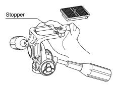
Remove the quick release platform turning the lock lever. In this case, please do not put the lock lever back by force as it has been stood by the stopper.
