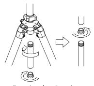
Remove the center column base stopper. Then remove the lower part of center column. Put the center column base stopper in from the upper part of center column.
