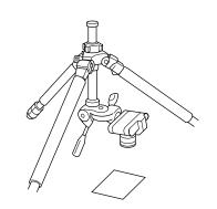
By inverting the center column, it is possible to do copy, and close up work.
