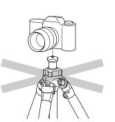
Do not attach camera directly to the threaded post of the center column. This may damage both of camera and tripod.
