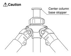
Always be sure to return the center column base stopper back on the center column. This prevents the center column pulled out accidentally.
