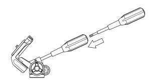
Remove the vertical tilt handle from the panhead, and screw into the back of the pan & tilt handle.
