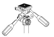
When tilt friction control knob is locked and pan handle is loosened, a friction of the vertical movement is increased. When pan friction control knob is locked and pan handle is loosened, a friction of the horizontal movement is increased.
