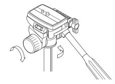
Lock the panning lock knob, then grasp the pan handle and turn the head, counter-clockwise to loosen.
