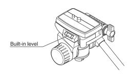
Adjust the built-in level to fit into the middle.
