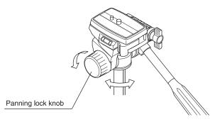
To rotate the camera left or right, loosen the panning lock knob. When you want to lock in at a certain position, tighten the knob.
