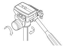
Set the pan head on the tripod's threaded post, and turn clockwise until it comes to a stop. Tighten the panning lock knob and turn clockwise slightly more.
