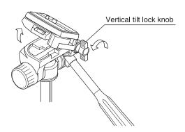
For vertical position shots with your still camera, loosen the vertical tilt lock Knob, and tilt the camera platform to the desired position. Then lock the vertical tilt lock knob.
