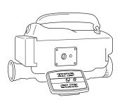
The retractable camera positioning pin enables you to mount both a video camera and a still camera.
