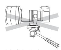
This product has been designed to handle equipment weighing under 1.5 kg (3 lbs 5 oz). Do not overload.
